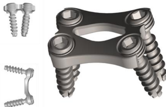
Figure: Representative illustration of the “half-hole” surgical plate with fastener and screw assemblies
